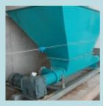
**Solid Fruit and Vegetable Waste** needs to be macerated and transformed into a pumpable solution. A customized Twin Shaft Auger with Pre-Macerating Effect feeds the material to the Multicrusher (not pictured) for further solids reduction. A Rotary Lobe Pump (not pictured) transfers the fluid (app. 15-20 % DS) to a storage tank.
