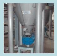
**Food Waste** often is used for animal feed or as substrate in anaerobic digesters. The Multicrusher increases surface area and therefore has a positive effect on retention times in the digestion process. Particle size is determined by the blade and cutter design and can be modified by rotation speed variation. In this case the Multicrusher is side mounted with a hopper on the suction side for easier food waste penetration into the macerator.
