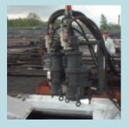
**Mixtures of heavy viscous waste oil,** water and solid waste need to be discharged out of a lined lagoon. A hydraulically driven combination of Multicrusher and Rotary Lobe Pump in submersible set up takes care of the job.
