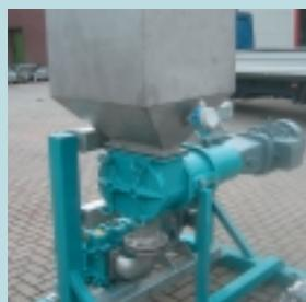
**Slaughterhouse Waste** needs to be macerated and transferred. A customized package includes a receiving hopper, a side mounted Multicrusher with increased suction opening and a Rotary Lobe Pump. The system is extremely compact, but still easy to maintain with Boerger MIP-Design.
