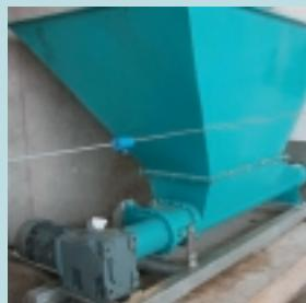
**Solid Fruit and Vegetable Waste** needs to be macerated and transformed into a pumpable solution. A customized Twin Shaft Auger with Pre-Macerating Effect feeds the material to the Multicrusher (not pictured) for further solids reduction. A Rotary Lobe Pump (not pictured) transfers the fluid (app. 15-20 % DS) to a storage tank.
